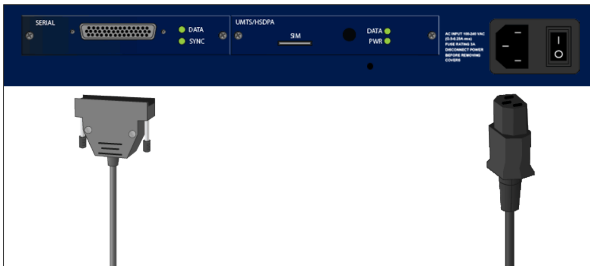
Figure 3: Serial and power connections on the rear of a GW9000 series router
