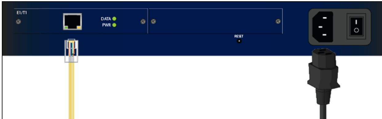
Figure 10: The cables you need for an E1/T1 and power connection
