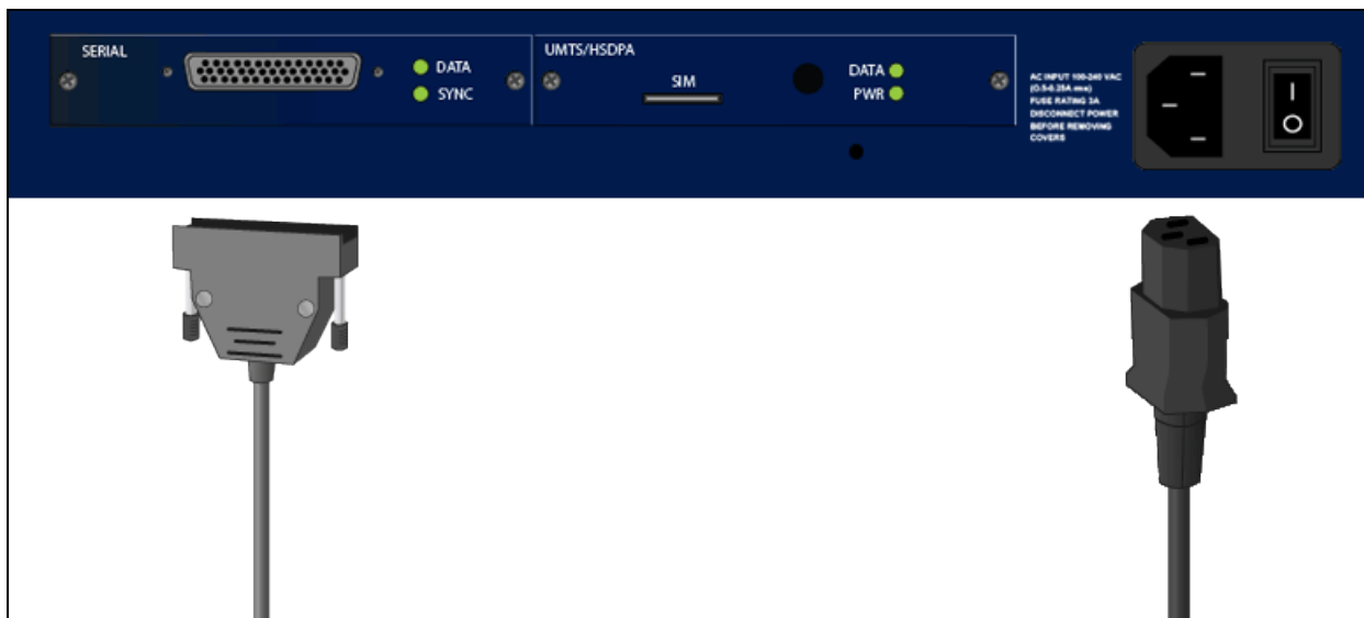
Figure 9: The cables you need for a serial and power connection
