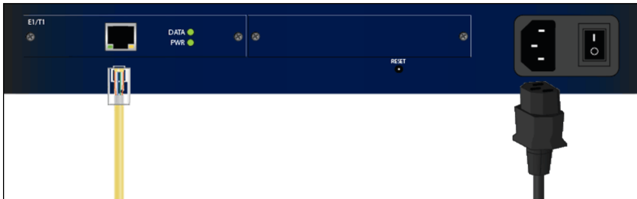
Figure 4: The cables you need for an E1/T1 and power connection
