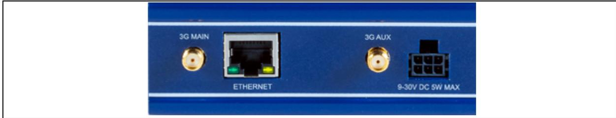
**Figure 3: Ethernet LED activity on the rear of a GW2021 router**
