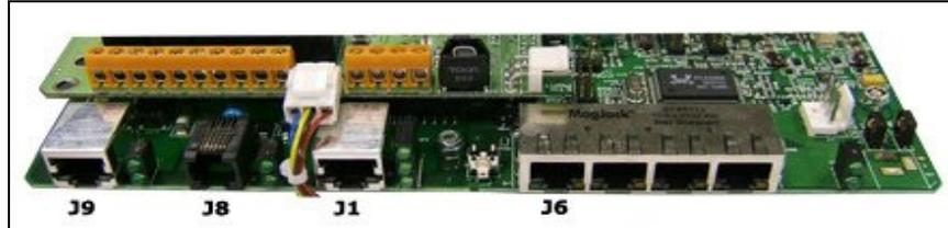
Figure 3: The ports on the ADSL board in the GW8600 SMG
