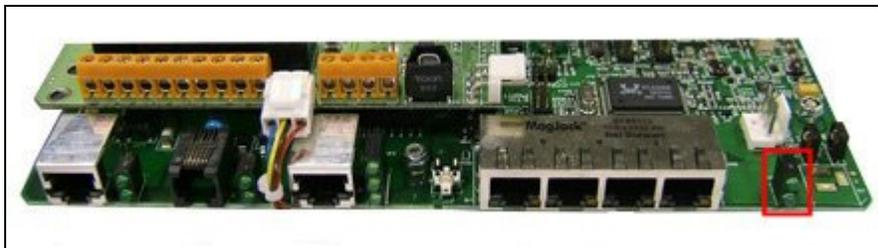
Figure 4: The power and configuration LEDs on the GW8600 SMG
